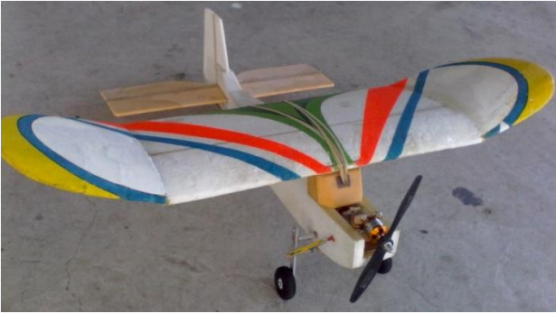
Norm Rodger's Lazy Bee with "Fieseler Storch" type undercarriage.
