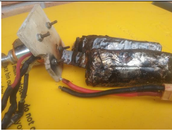
This is what happens if your engine bolts are too long and your plane stops suddenly!
