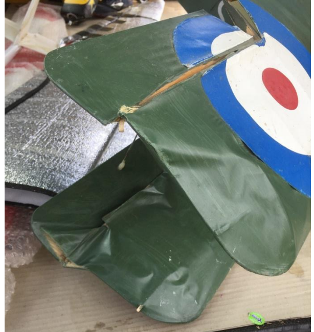
Ian McEwan's (niece) SE5 after losing elevator control due to plastic horn breakage. A message here to all flyers! Check your control linkages more often and replace them, especially plastic as it goes brittle pretty quick! Ian's SE5 was 25 years old, so amazing it lasted that long!
